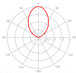
V/H - Port Pattern Azimuth 5.6 GHz
