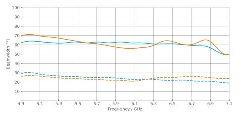
Beamwidth Azimuth H - 6 dB
