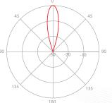
V/H - Port Pattern Azimuth 5.5 GHz
